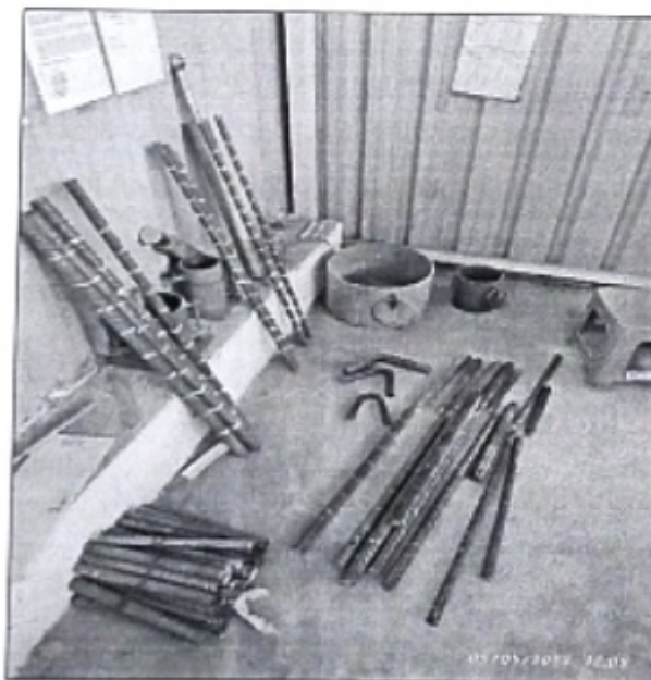
Image3-Materials to be tested (TMT Bars)
